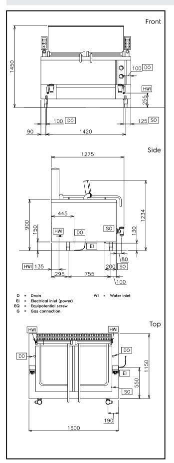
**Electric** Supply voltage: 291161 (CR42G) 230 V/1N ph/50 Hz Gas Gas Power: 60 kW Gas Type Option: LPG; Natural Gas Gas Inlet: 1"1/4 **Key Information:** Number of wells: 2 Usable well dimensions (width): 625 mm Usable well dimensions (height): 410 mm Usable well dimensions (depth): 640 mm 190 It MIN; 190 It MAX Well capacity: External dimensions, Width: 1600 mm External dimensions, Depth: 1280 mm
